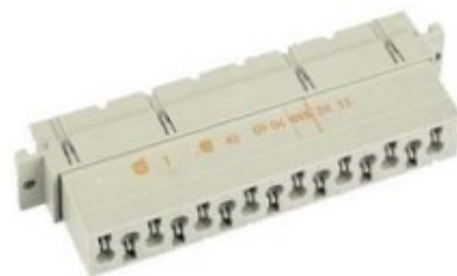
Figure 11. Standard with N-mechanics H15 Cage Clamp type female - H15-CC . The cable rating is AWG16 or <1.5 \text{ mm}^2 . That makes it not usable for 24T-input and 5 V outputs.
