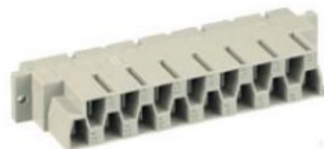
Figure 12. Optional H15 FastOn 6.3 mm female N-H15-T. The TABS are rated 12 A 70°C or 15 A 55°C thus 2.5 \text{ mm}^2 or AWG13
