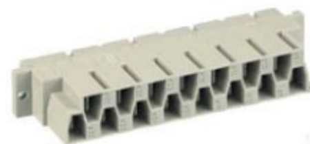
Figure 10. Optional connector H15 FastOn 6.3 mm female N-H15-T The TABS are rated 12 A 70°C or 15 A 55°C thus 2.5 \text{ mm}^2 or AWG13
