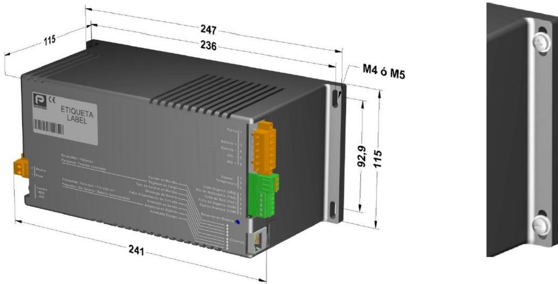
Figure 1.- Device installation position (NP-0719 and NP-0716)
