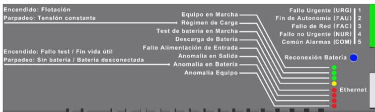
Figure 16.- LED and relay position
