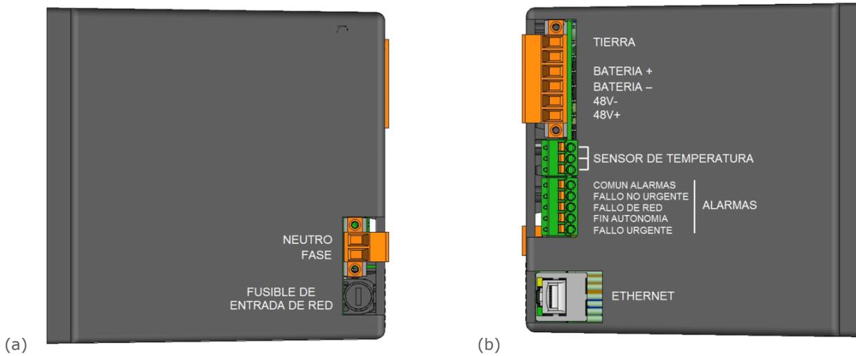
Figure 3.- Models NP-0716 and NP-0719. (a) Left side view and (b) Right side View
