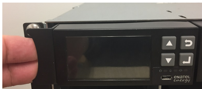
Figure 10: For removal, pull the controller forward
