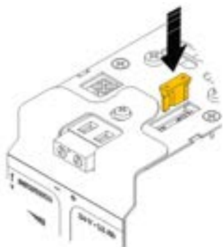
Figure Error! No text of specified style in document. 12 – BBX Battery box: a) Removing and b) Inserting fuse.
