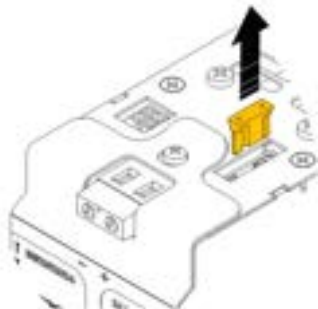
Figure Error! No text of specified style in document..27a – BBX Battery box Removing fuse.
